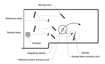
Figure 3: Angular accessory principle.
