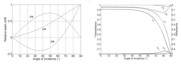
Figure 2: (a) relative beam shifts in function of incidence angle, (b) amplitude of multiple components in function of incidence angle.
