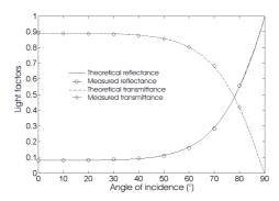
Figure 5: Comparison between theoretical model and experimental results for a clear glass.
