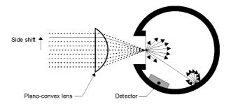
Figure 4: Positioning of plano-convex lens.
