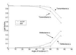
Figure 6: Comparison of light transmittance and reflectance factors between ADOPT Project and BBRI results.
