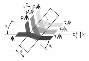
Figure 1: Multiple reflections in a simple glass sheet
